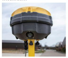
Intellicam is a portable incident camera that captures site incursions, customer confrontations or any other activity in and around a work site, giving workers an extra layer of protection and providing stakeholders with specific, relevant data and evidence when needed.
